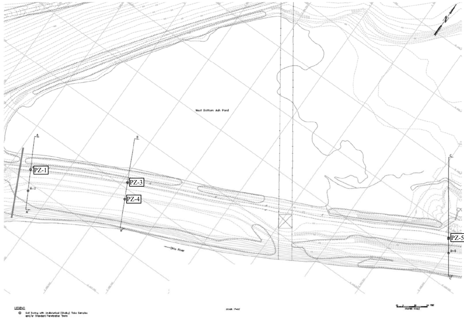
FIGURE 1. WEST BOILER SLAG POND PIEZOMETERS LOCATION PLAN
